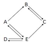
Figure 1. Reaction mechanism of dissolution of gibbsite and transformation of kaolinite to DSP. A: kaolinite, B: dissolved silica, C: sodium aluminium hydrosilicate (DSP), D: gibbsite, E: dissolved alumina
